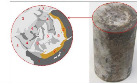
Laboratory tests on core samples- different compacted solids (salt, bentonite, barite) in different states
